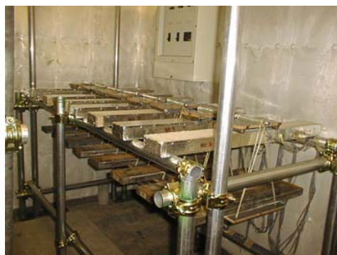
Sustaining loading test
